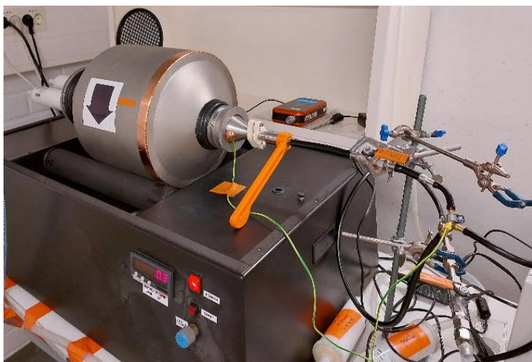
Figure 1. The dustiness test set-up.
